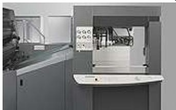
The automatic non-stop unit considerably facilitates pile change as all functions can be easily activated at the push of a button without the need for manual intervention. In combination the Logistics system, pile change is initiated automatically as soon as the pile height falls below a certain pre-defined level.
