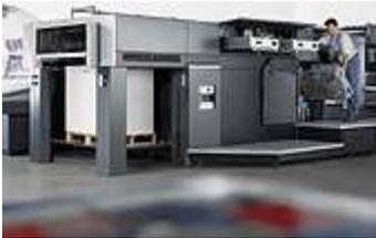
and the powder spray device can be completely controlled from the CP2000 Center . All major air and format settings can also be performed conveniently on the CP2000 Center or the operating panel on the delivery. Its
