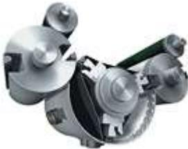
The patented Air Transfer technology makes the Speedmaster CD 102 the ideal press for serving wide range of printing stock. The blast air is blown outward from the middle of the press by Venturi nozzles. This generates a cushion of air on which the sheet rides while smoothly adapting to the shape of the sheet guide plate. The Air Transfer System is controlled by the CP2000 Center - simply, quickly and with absolute precision - ensuring non-smear print results even at top press speeds.
